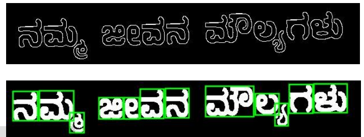
Figure 6: Canny Edge and Rectangular Bounding Boxes
