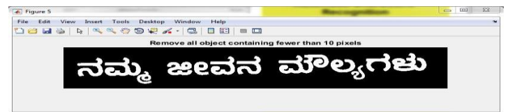
Figure 13: Removing Unwanted Objects less than 10 pixels
